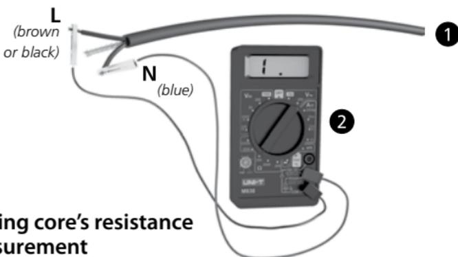
**Heating core's resistance measurement**
